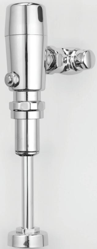
**Hygiene Flush:** To maximize hygiene, this product is equipped with a 24 hours duty flush. The flush takes place after 24 hours of non use have passed. Prevents the trap seal from drying out, possible freezing of pipes, and gets rid of potential bacteria in stuck water. This function can be disabled using the remote control.
