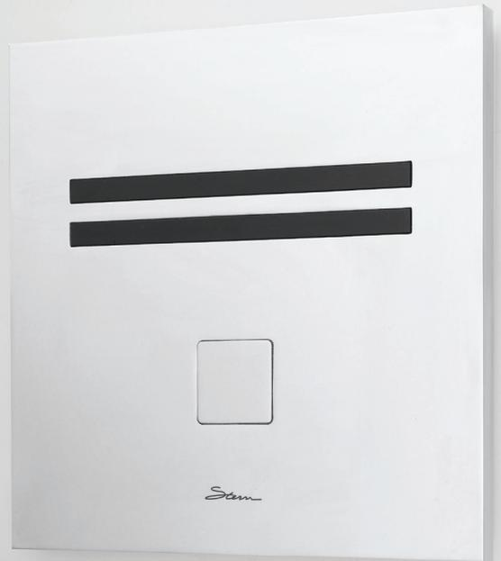
**Hygiene Flush:** To maximize hygiene, this product is equipped with a 24 hours duty flush. The flush takes place after 24 hours of non use have passed. Prevents the trap seal from drying out, possible freezing of pipes, and gets rid of potential bacteria in stuck water. This function can be disabled using the remote control.
