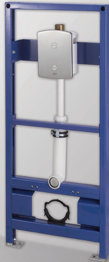
**Hygiene Flush:** To maximize hygiene, this product is equipped with a 24 hours duty flush. The flush takes place after 24 hours of non use have passed. Prevents the trap seal from drying out, possible freezing of pipes, and gets rid of potential bacteria in stuck water. This function can be disabled using the remote control.
